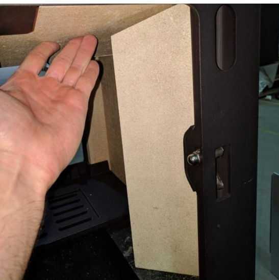
3: Lift the Baffle Brick to enable the removal of the RH Side Brick.
