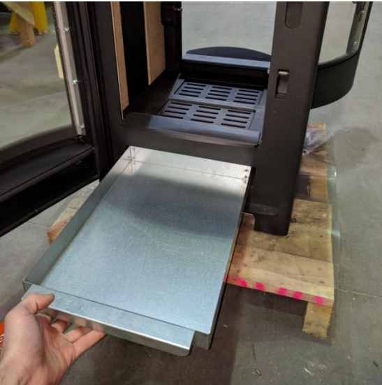
1: Remove ash pan; this makes it possible to push the grate up from beneath.
